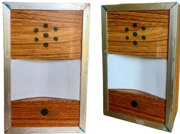
Figure 3: Prototype of a waterproof doorbell motion sensor.
